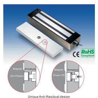
When there is no power, there will be no holding force, and the push-off button will pop out immediately, to release the Electromagnetic Lock and the Armature Plate for no residual magnetism.
